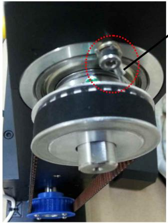
1. Please check whether the terminal of bolt is contacted with the axis of roll.
