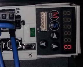
(The initial display of motor driver should be the state of (PRr000)
