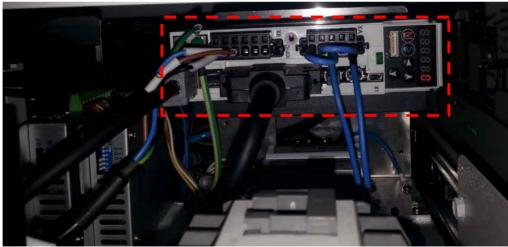
(There is the motor driver of roll at the right side inside the machine)
